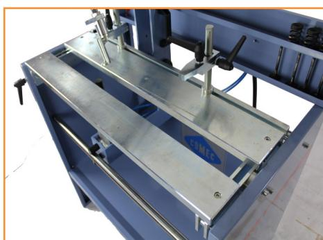
The BST860 cylinder head work station allows all kind of operations on cylinder heads as disassembling, reassembling and their all-around control in an efficient, practical and safe manner.
